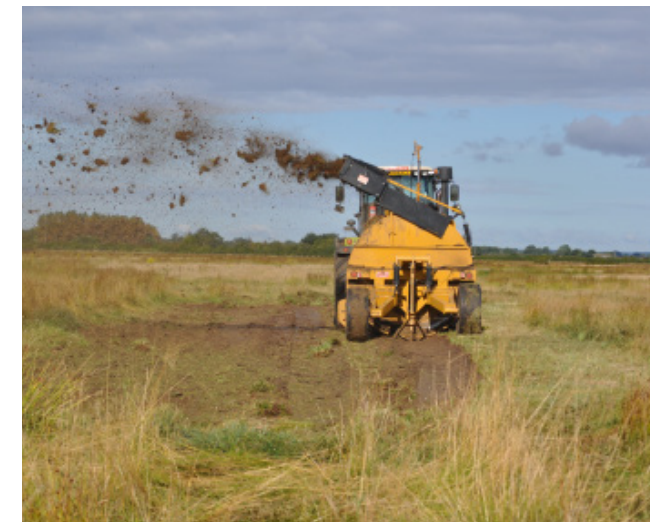
Rotary ditcher dispersing soil
