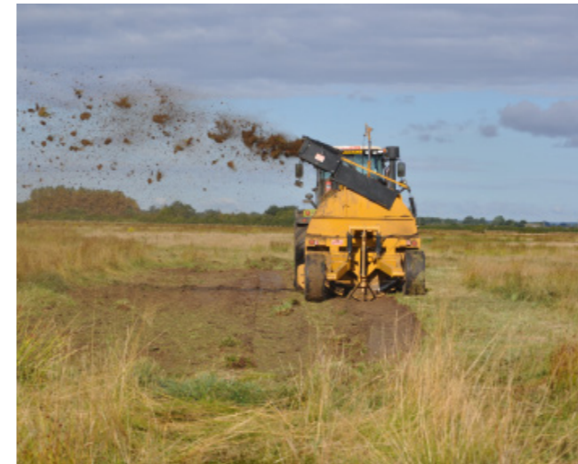
Rotary ditcher dispersing spoil
