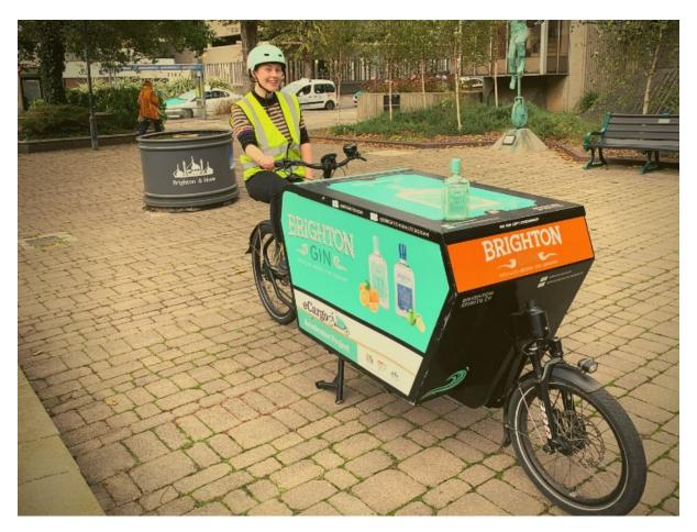
All the proposed vehicles have a 250W electric motor powered from rechargeable batteries to help with heavy loads and hills. We have trialled eCargo bikes on Wyle Cop to confirm that they are capable of the steepest hills we will encounter.
