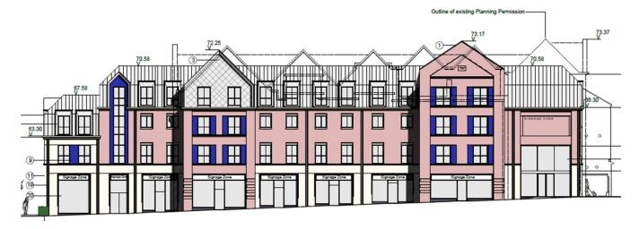
This illustrates that the application scheme is demonstrably lower than the extant scheme with a significantly lower eaves line. While it extends closer to Rowley's House than the extant scheme there remains a gap of some 10.5m and the architecture steps down and away from the frontage highlighting Rowley's mansion within Barker Street when viewed from the South.
